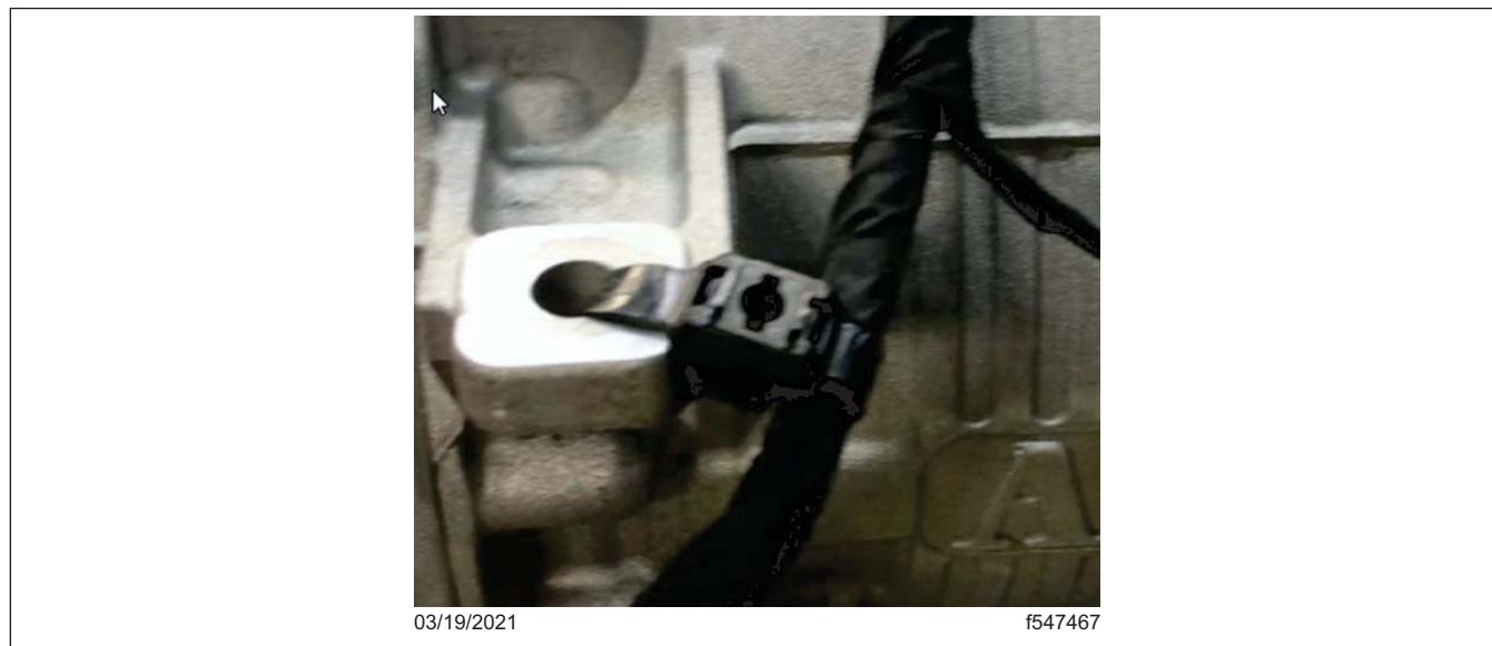
Fig. 10, Using a Butterfly Strap to Clip the Harness to the Transmission
