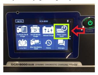
**CRITICAL:** Power Supply Mode voltage must be stabilized at **13.5** Volts before proceeding.
