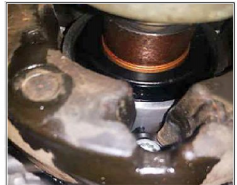
Oil leak on output-shaft radial shaft seal
