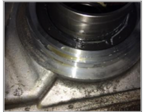
Oil leak on input-shaft radial shaft
