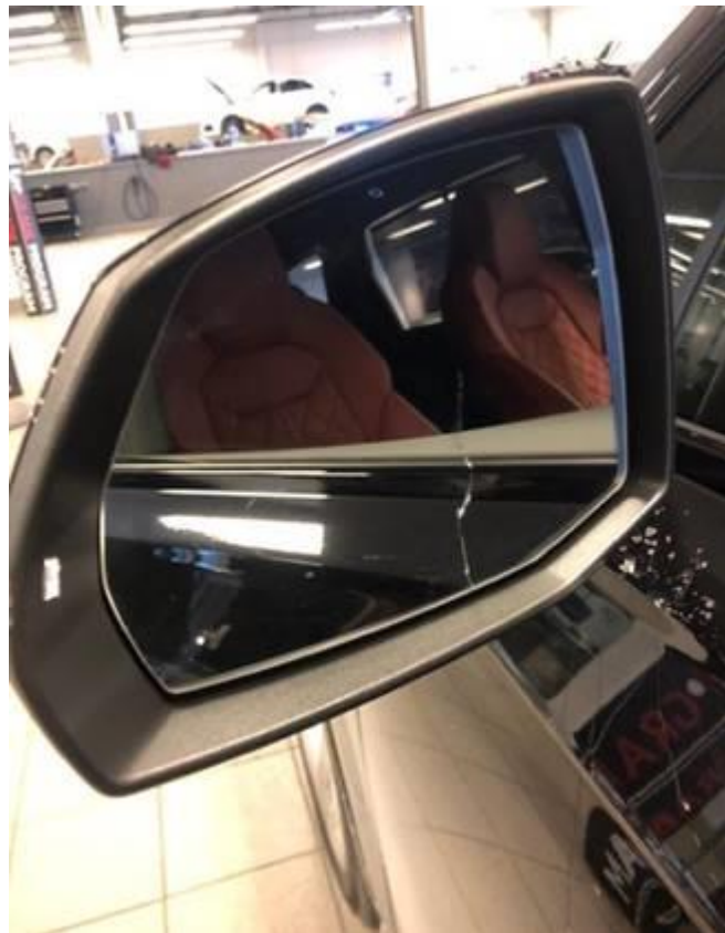
Figure 1. Exterior rear view mirror glass cracked.
