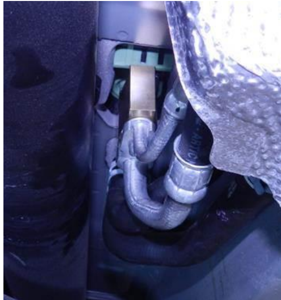
Figure 13. Location of rear air conditioning unit expansion valve.
