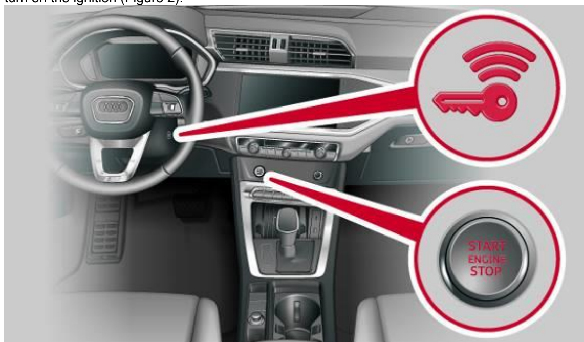
Figure 2. Key reader coil location.
