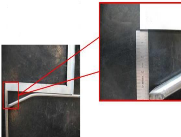
Figure 18. Verifying distance of 43mm in the bend.
