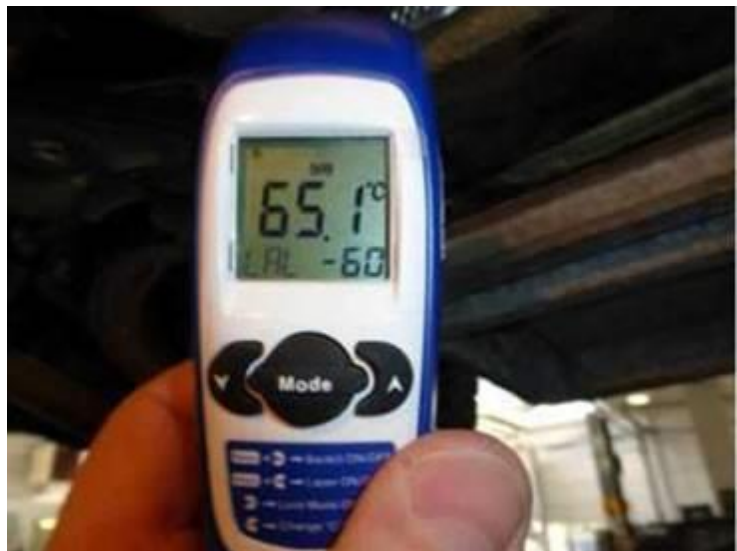
Figure 5. Surface temperature warmed to 65° C (149°F).
