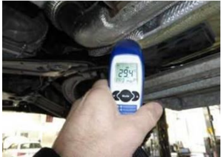
Figure 6. Surface temperature cooled to approximately 30° C (86°F).
