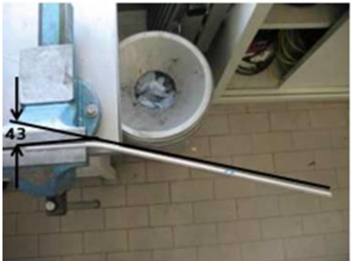
Figure 17. Bend created 43mm from the axis of the long end of the steel rod.
