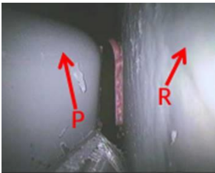
Figure 27. 3mm gap created between reinforcement plate and longitudinal member.
