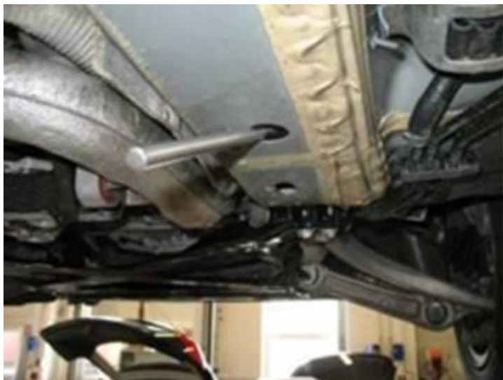
Figure 26. Steel rod driven forward at least 10mm.
