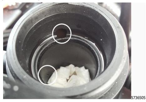
3. Stuff a shop rag or a paper towel into the radiator fill neck to prevent debris from falling in the coolant, as shown.
