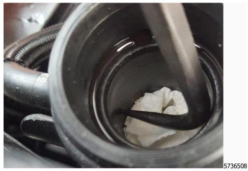
4. Using a radiator hose removal pick, poke through the vent port to clear out and remove any casting flash.
