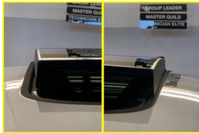
Figure 1. An opened sunroof glass panel in a 'twisted' state.
