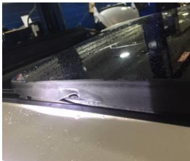
Figure 2. A distorted 'skirt' on the side of the sunroof glass panel.
