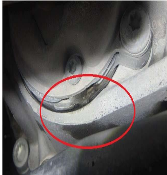
Figure 2. Oil leaking in area of the auxiliary hydraulic pump (V475) detail.
