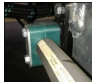
Figure 6. CORRECT Use of Hose Clamps for Hoses
