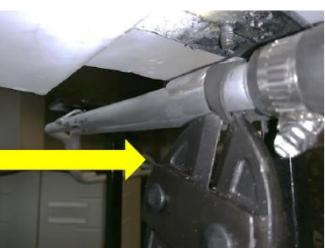
5. Using a bolt cutter, cut the spring-band clamp into 2 parts and remove it.
