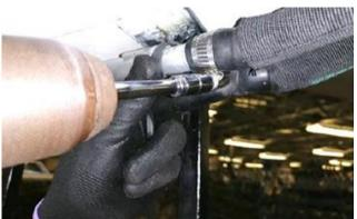
4. Secure the hose/pipe connection with a hose clamp, part number 64 21 8 367 179 and tighten to 4 Nm.
