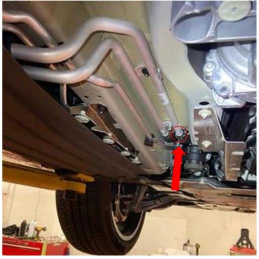
The aluminum pipe and the hose are connected to each other by a spring-band clamp.
