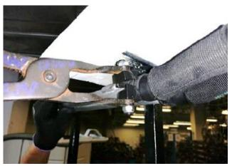
2. Open the spring-band clamp using special tool pliers 172050.
