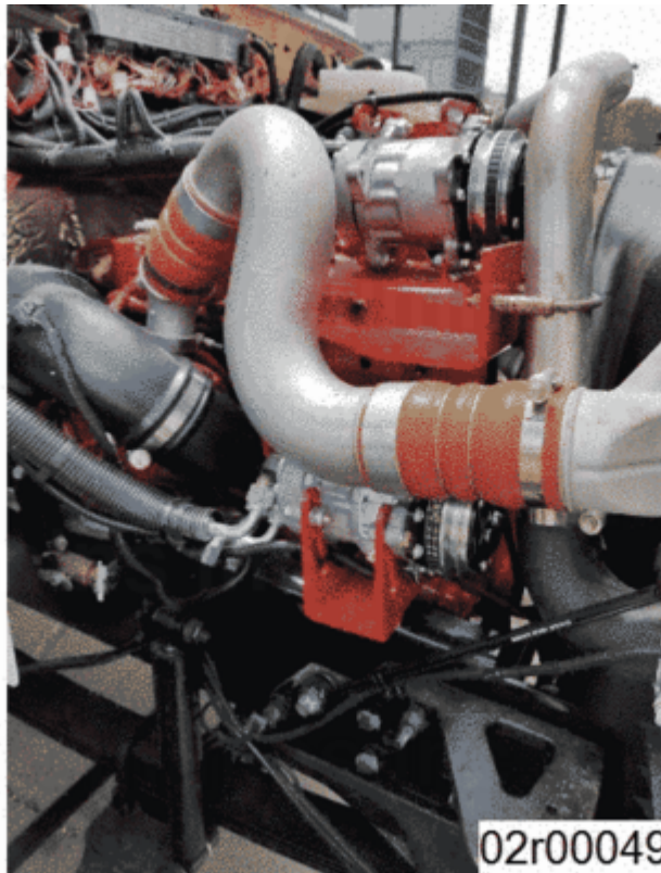
Figure 1, Non-Approved Bus Air Charging System Alternator Bracket.
