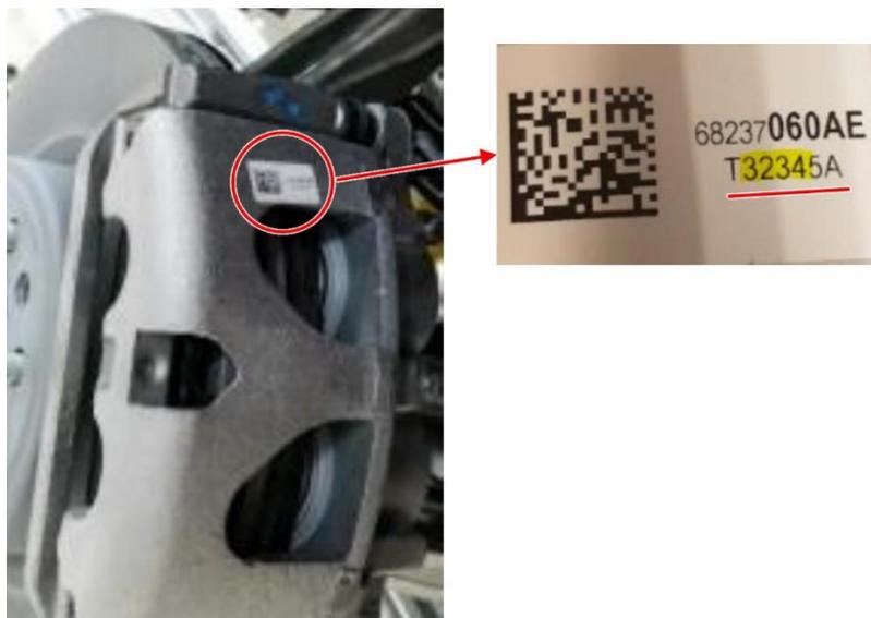
Figure 1 – Front Brake Caliper Part Number and Julian Date Code
