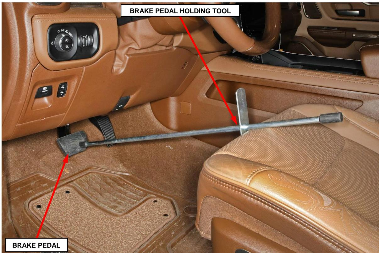
**Figure 2 – Brake Pedal Holding Tool**
