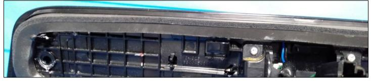
Check: once the CHSML is installed onto the vehicle there should be no gasket visible from the top or the sides.
