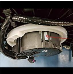
**4.5. Check for signs of a blueish tinge on the white plastic windows, as shown in the picture above, that indicate reductant contamination or oxidation and continue to the next step.**
