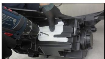
6. Remove the jig, and slowly drill into the pilot hole using the larger drill bit 20 mm (25/32 inch).
