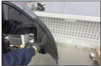
10. Insert a flat-head screwdriver into the hole to inspect the headlamp.
