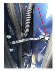
• Using the plastic trim tool, insert between the door frame and weatherstrip then twist it to release the 2 molded-in weatherstrip retaining clips as shown below. One clip is located at the top rear corner, the other in the top front corner.
