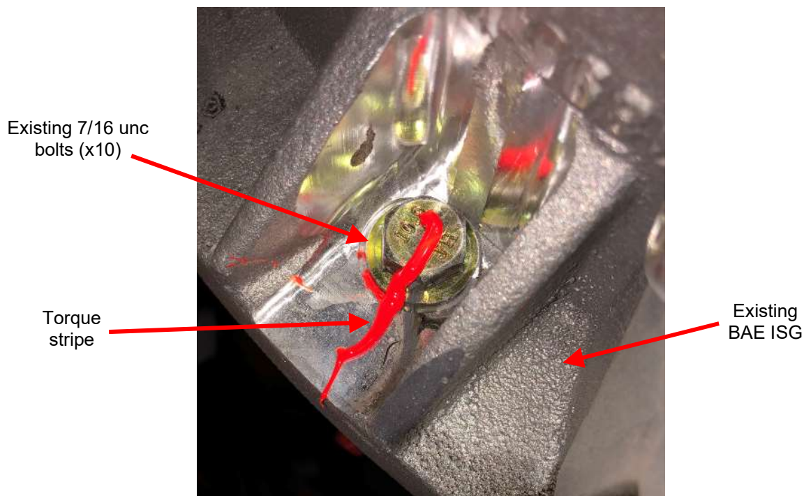
Figure 3: Pictorial of Correct Bolt Torque Stripe
