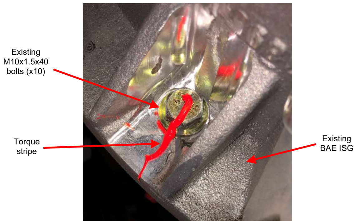
Figure 3: Pictorial of Correct Bolt Torque Stripe
