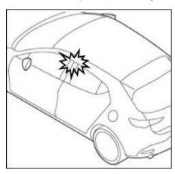
Since the front door glass run channel is not fixed to the door strongly enough for the following situations, cycles of door operation may result in interference and lead to damage on the seal rubber at the rear door.
