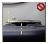
Metal bracket recesses are not aligned to the corresponding indicators on the rubber part.
