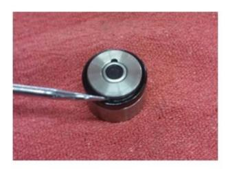
**6.** Lubricate the piston and the new U-cup seal lightly with silicone grease to ease installation. Slide the new U-cup seal over the piston, ensuring the cup faces away from the piston as shown.
