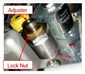
**13.** Verify that with the fuel pump running, no fuel leaks are noted from the atomizer. Exit the diagnostic session in the DX2 and turn the ignition off. Do not disconnect the DX2 at this time.
