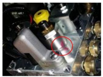
2. To allow a socket to be placed over the fuel pressure regulator housing for removal, it will be necessary to loosen the air solenoid retaining nut located above the fuel pressure regulator and rotate slightly. Refer to the photographs below, which show a view of the atomizer from above, for reference.
