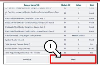
This screen will confirm KDS has successfully electronically transmitted the vehicle's IUMPR data to Kia's server.
