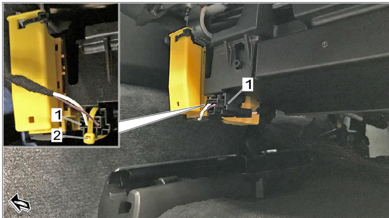
Electric plug connection for front seat ventilation
