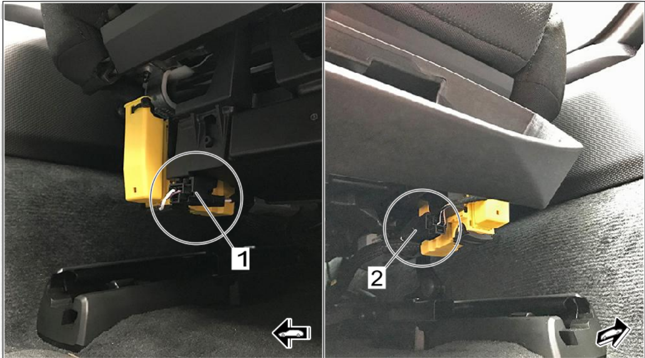
Plug connections for front seat ventilation
