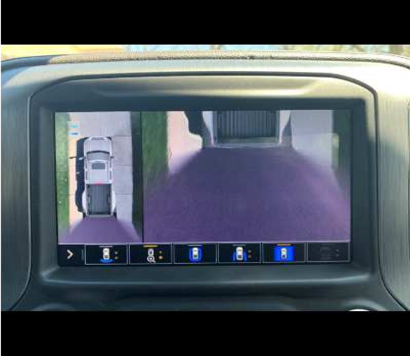
Tailgate overhead camera, Tailgate removed
