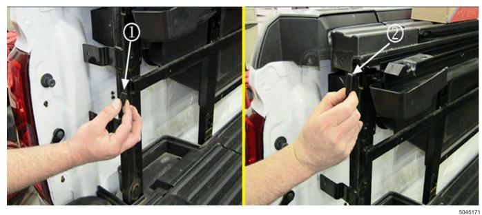
**Note:** A short lower (1) and a long upper (2) plug will be installed at the rear. Only a short lower plug will be installed at the front.
