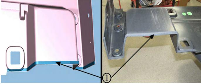
**Note:** To improve tape adhesion, clean the plastic surface of the pickup box side liners using Kent Automotive Acrysol, or a suitable solvent, prior to the tape application.
