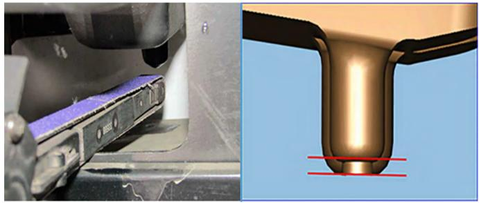
**Note:** Because of the limited vertical access to the front drains, enlarging the front drain opening is attained by removing material from the bottom of the drain.
