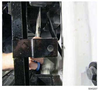
**Tip:** Using needle nose pliers, or a suitable tool, will aid in tightening the tie strap.
