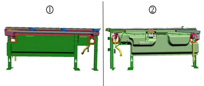
**Note:** The illustration above shows the right cargo stow bracket in vehicle position (1) and removed showing the backside (2) to clearly show the drain/hose locations. It is not necessary to remove the stow bracket to complete this repair.
