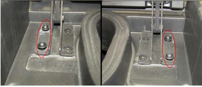
18. Tighten the 2 most forward and 2 most rearward bolts on both the left and right side tool box lid hinge springs.
