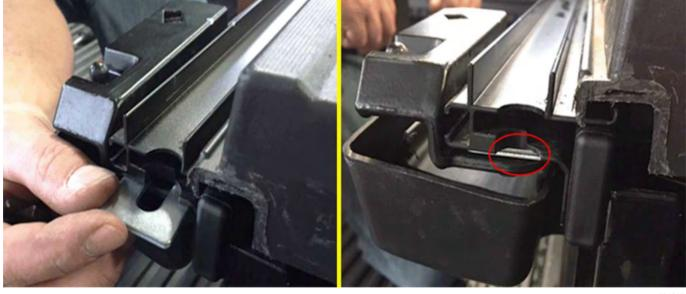
**Note:** Installation of the right rear shim is shown in the graphic above.
