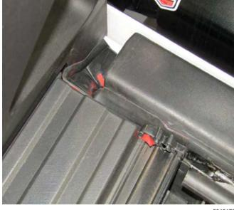
15. Without removing the red adhesive backing tape film, dry fit the new left and right front pickup box liner insulators (muckets) into position.
