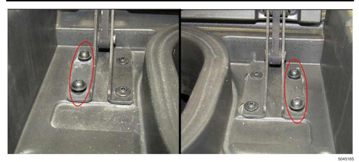
**Important:** ONLY loosen the 2 most forward and 2 most rearward bolts on each side. This prevents mis-alignment of the tool box lid upon re-assembly.
