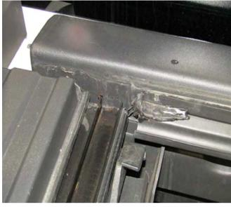
9. Remove and clean off any remaining tape residue, or sealer, at both insulator locations. Final clean both locations using Kent Automotive Acrysol, or a suitable solvent.
