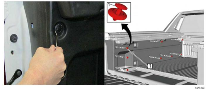
**Tip:** To ease removal of each retainer, insert a pick, or other suitable tool, into one of the 3 openings of the retainer center, and pull to disengage the center portion completely.
