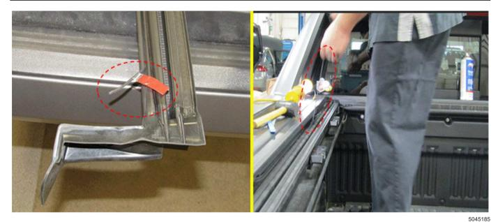
16.5. Pull the release string off of the new seal from rear to front, to seat the inboard lip of the seal into position.
