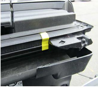
**Note:** The side pickup box cover seal is shown installed in the graphic above for illustration proses only. The seal will actually not be installed until a few steps later in the repair procedure.
