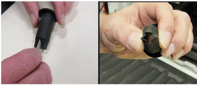
11. Using a razor blade, or suitable tool, cut slots into the bottom opening of each of the 4 drain plugs.
