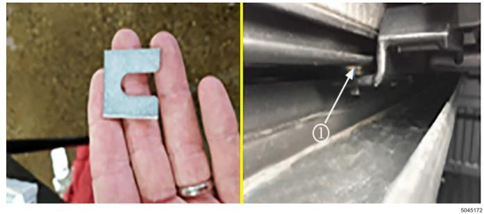
**Note:** The addition of shims under the latch brackets will increase the load force on the closed latch.
