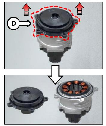
7. Check for coolant intrusion and terminal corrosion in the AEWP housing and take action according to the procedure and example photos.
