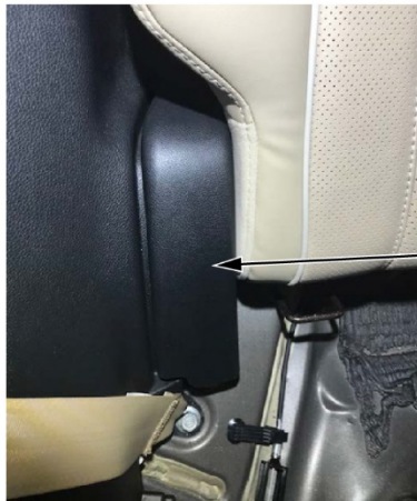
SEAT HINGE COVER Lift up.
