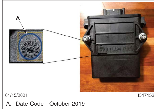
Fig. 4, TPMS Housing Date Code
