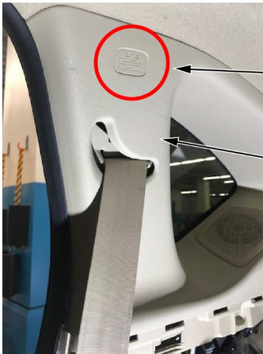
Lightly tap this area with a rubber mallet.
