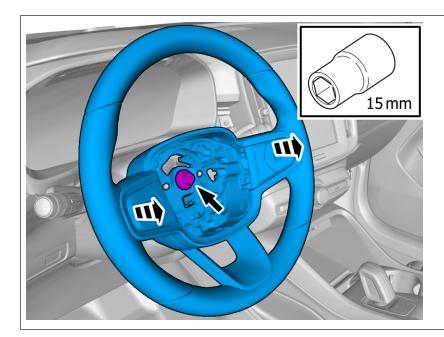
Loosen the screws. Remove the marked part.
