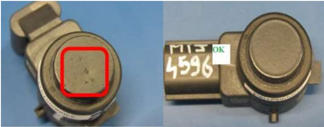
Figure 5: signs of impact on the parking sensor.
