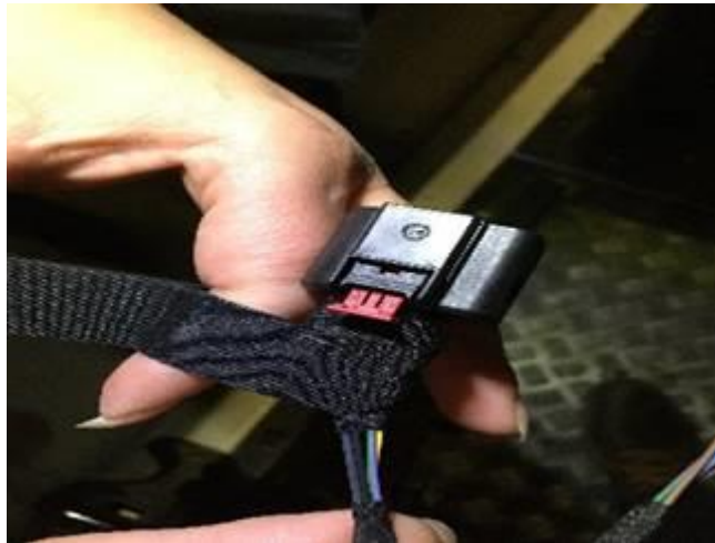
Figure 4. Wrapping the connector base part 2.
