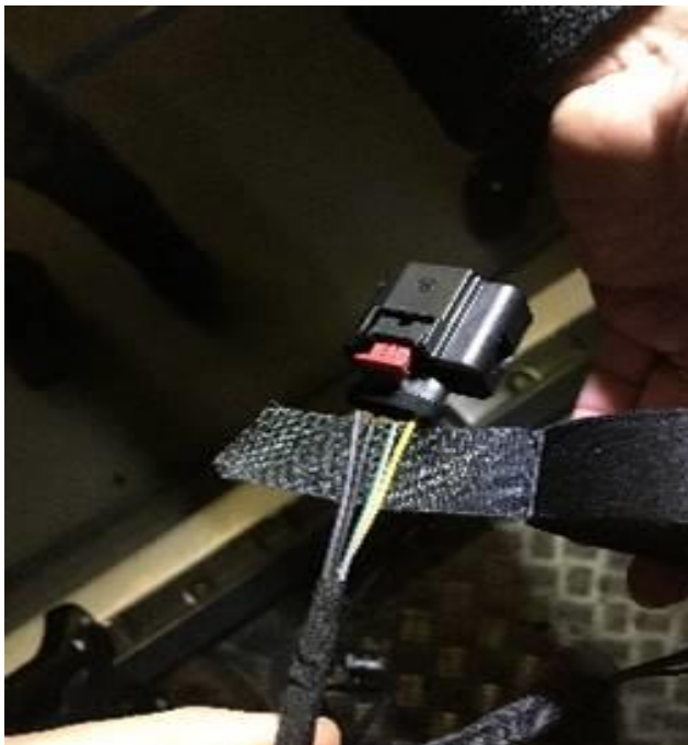
Figure 1. Wire is broken at G31 sensor.
