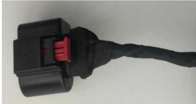
Figure 5. Completed harness wrapping.
