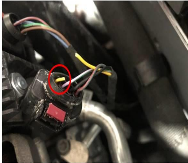
Figure 1. Wire is broken at G31 sensor.
