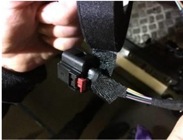
Figure 3. Wrapping the connector base.
