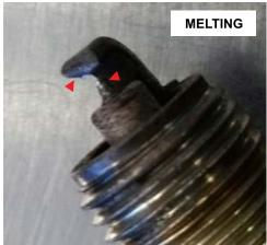
**NOTE:** Any damage to the spark plug porcelain outside of the cylinder head is not a result of this condition.
