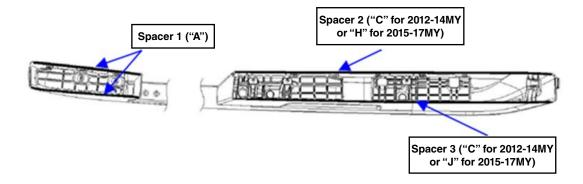
• The new cushions need to be within .5 mm of the inside of the molded-in guide lip but not overlapping onto or covering it. See **Figures "A" and "B"** below for reference.
