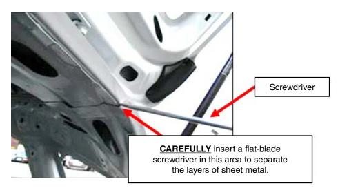
• After separating the layers of sheet metal, SPARINGLY apply a SMALL amount of the Endura penetrating grease into any newly-created gap using the aerosol applicator tube to be more precise and eliminate any overspray.
