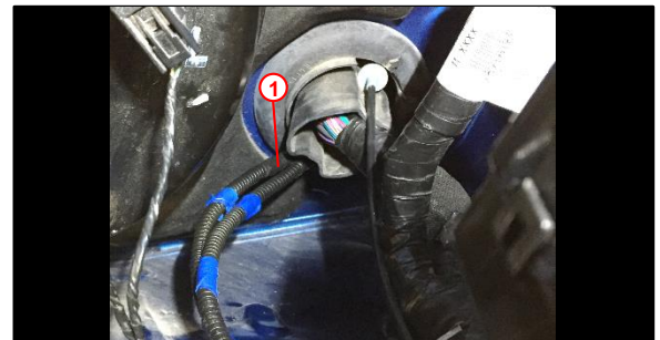
1 Engine Compartment – Corrugated Sub-wire Harness Covers
