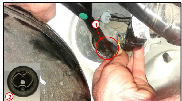
1 Cut at Grommet Indent Mark 2 Modified Grommet
