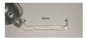
Apply grease to the serrated areas using a clean screwdriver or similar tool.
