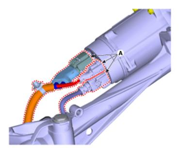
2. Remove the mounting clip (A), then replace the lead wire.
