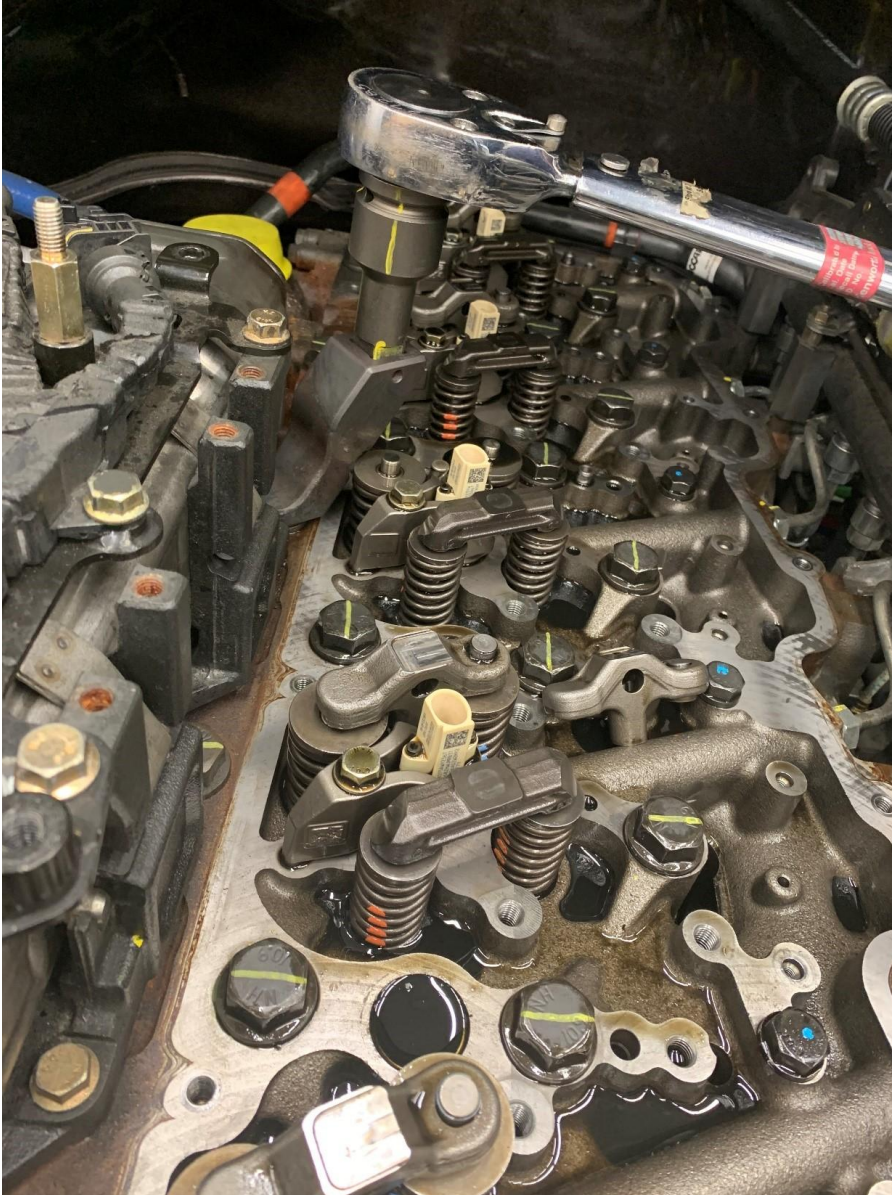
Figure 2 Example of Index marks and using the torque adapter tool
