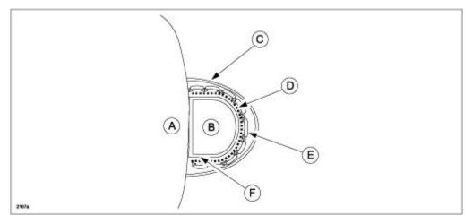
**NOTE:** Ensure the aluminum foil tape (F) is inserted into the edges of the molding (B) as shown below.
