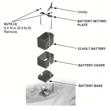
4. Remove the battery, battery cover, and battery base.
