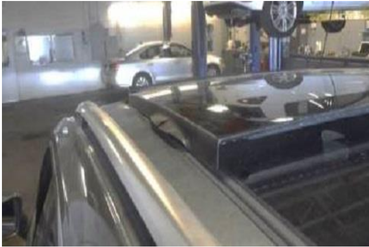
Figure 3: Example of the sunroof panel molded seal warped/deformation.
