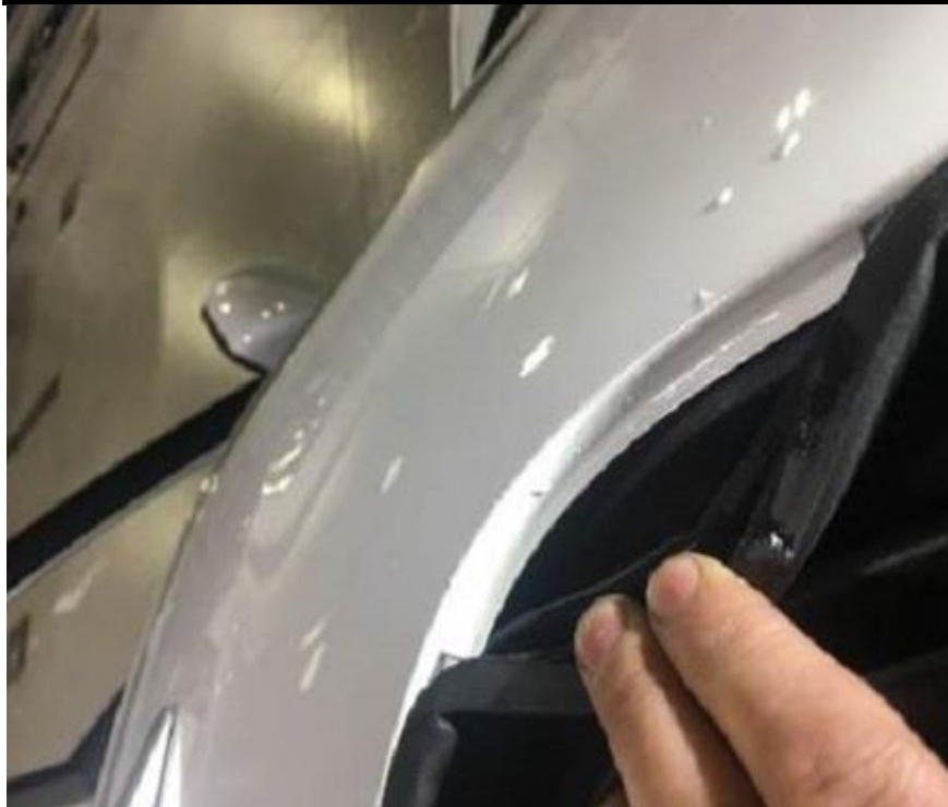
Figure 2: Example of the sunroof body side seal not having proper adhesion to the body.
