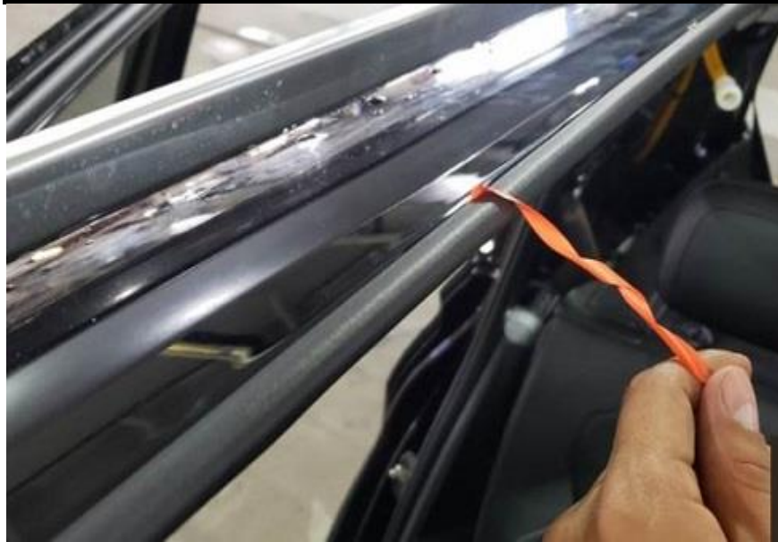
Figure 6: Example of removing the “red” protective tape after seal has been properly seated.
