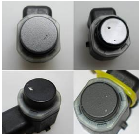
Figure 3. Stone chips causing sensor failure.
