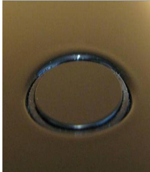
Figure 10. A correctly installed parking aid sensor.
