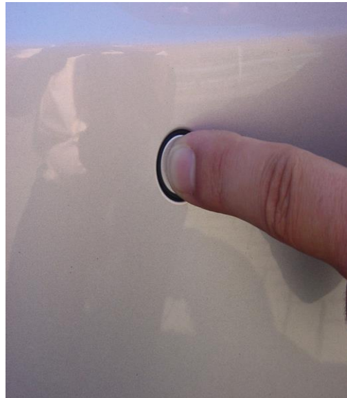
Figure 4. A pressure check on a parking aid sensor.
