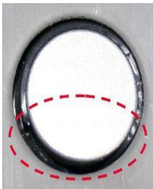
Figure 7. An incorrectly seated decoupling ring (folded).
