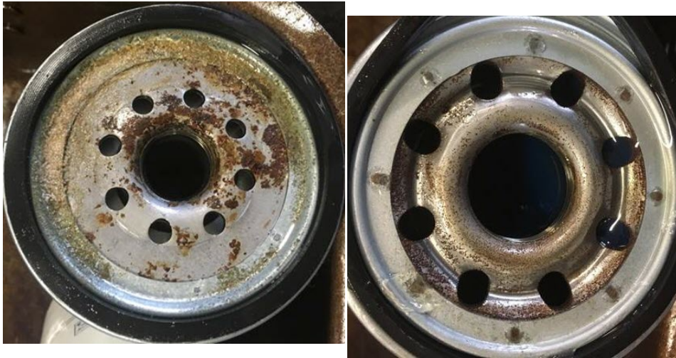
Crystal buildup and corrosion/rust present on primary filter
