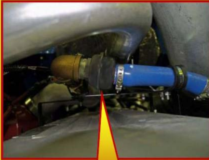
DPF Combustion Air Check Valve
