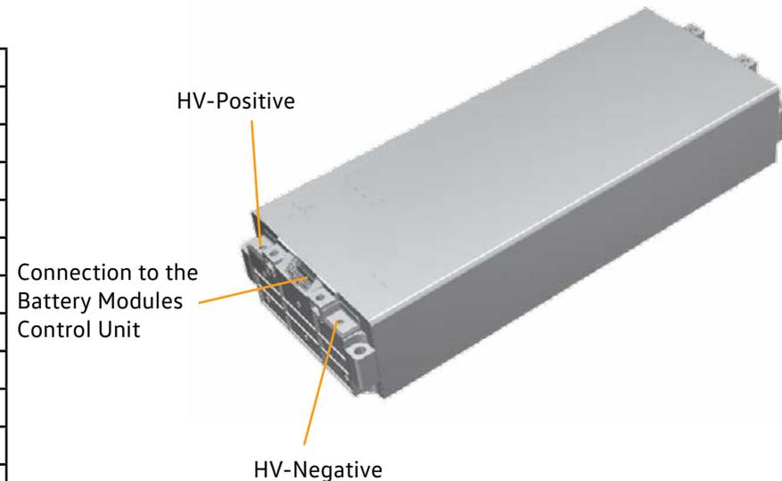
62 kWh Battery Module
