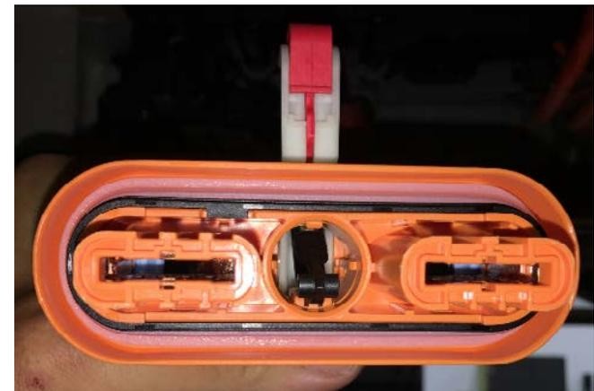
To ensure that the contacts still have the necessary cross-sections, the connectors are wide.
