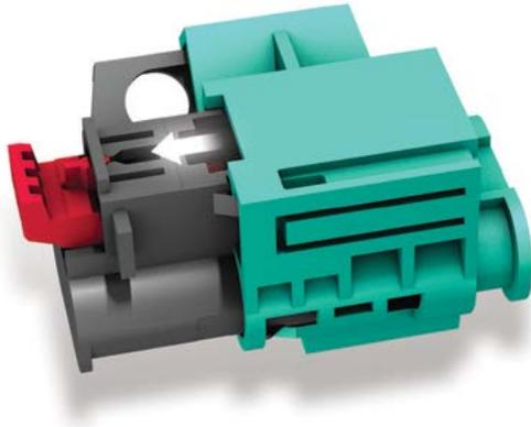
The fuse SC28 has a small “flag” on it. When removed, terminal 30 A is disconnected. The small “flag” is attached to allow quick removal without tools. The small “flag” can be replaced separately and the fuse is commercially available.
