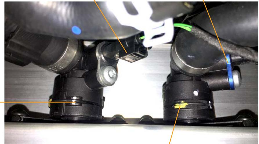
High-Voltage Battery Coolant Inlet
