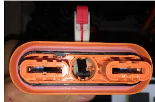
Shielding of the high-voltage wires is not required. The EMC measures are implemented in the high-voltage components by the EMC filter.
