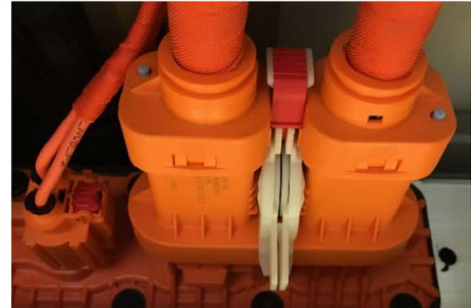
All HV wires in the ID.4 are connected mechanically. No screw connections on the wires are used.
