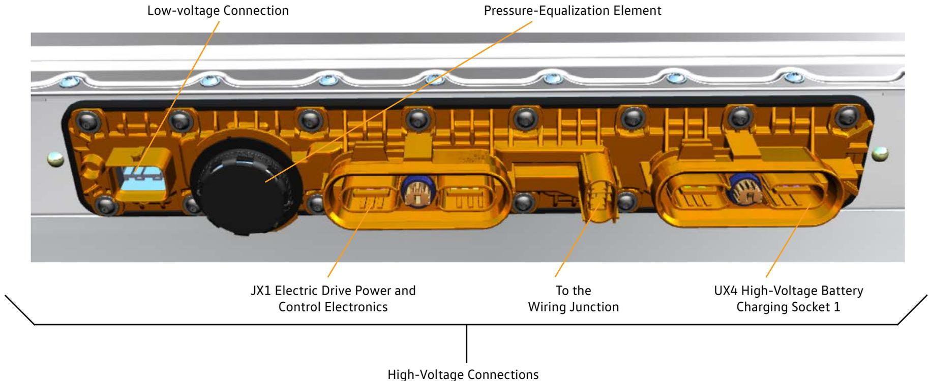
Assignment of the low-voltage connection T32g:
