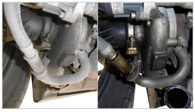
Oil leak on right turbocharger
