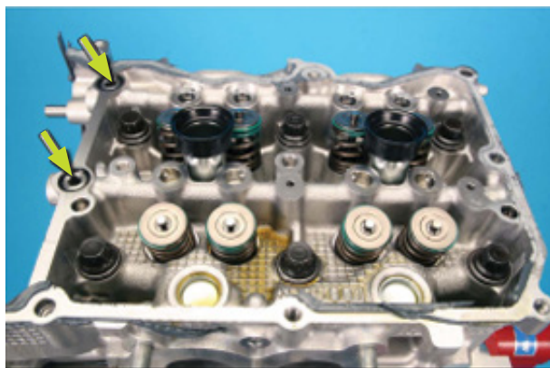
One-time use cam carrier o-rings which must be replaced.
