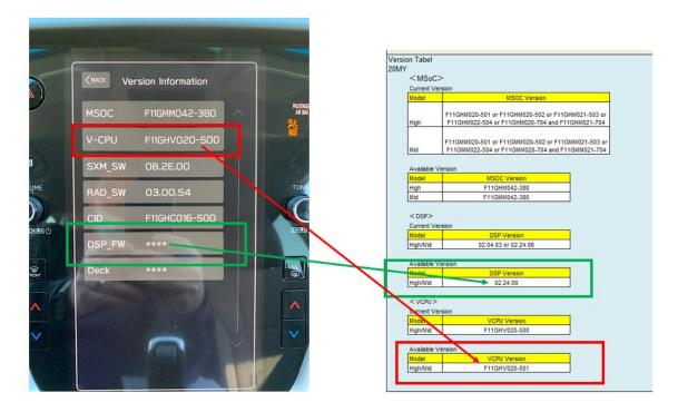
If the version displayed for MSOC is incorrect or there is no "RAD\_SW" version and "DSP\_FW" version displayed or asterisk symbols (\*\*\*\*) are shown, the software was corrupted during the software update. Should this occur, **NEVER** use the same USB drive for another update without reformatting it and loading a new set of the update files as outlined in the related service bulletin.
